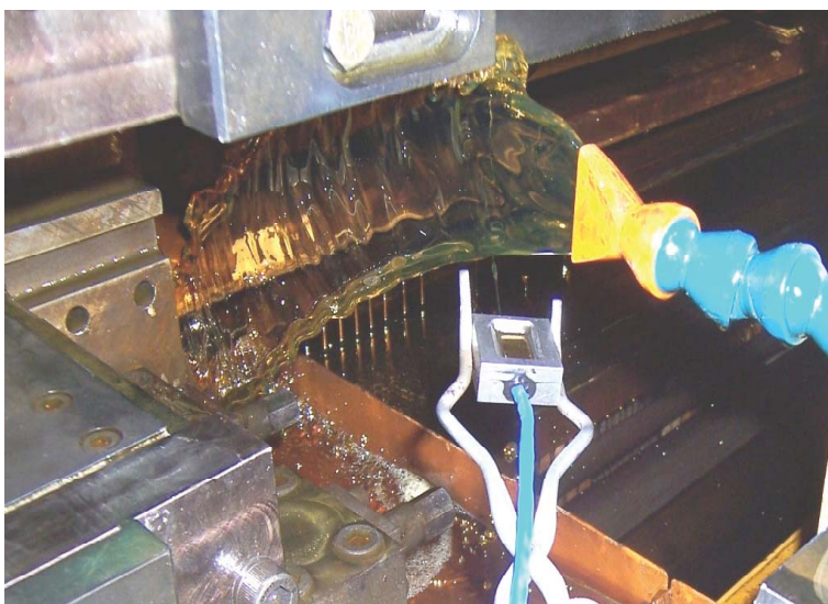
Figure 1: An acoustic sensor instantaneously measures the viscosity of cutting oil being used on a spline rolling machine. Changes in viscosity are indicators that the cutting oil may not be functioning as required.
